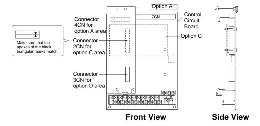
**Note** When the CompoBus/D Communications Card is mounted, other Optional Cards cannot be mounted in the C area.
